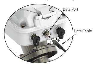
Figure 5. Attaching The Data Cable to the Mc Mag 3000
