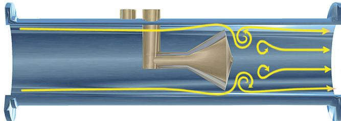
The contour-shaped cone directs the flow away from the cone, keeping the beta edge free from wear. Therefore, V-cone flow meters rarely require recalibration or replacement.
