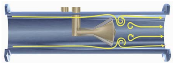
Figure 3: The V-Cone Redirecting Fluid Around The Cone
