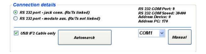
About the converter connection cable, ISOCON is set with "USB IF2 Cable only"; if the customer does not use the IF2 cable, this flag must be deselected.
