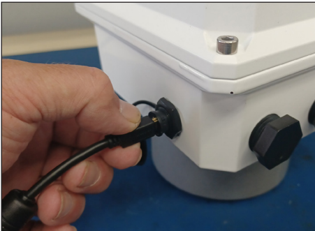
Figure 51. Plug in mini-USB cable
