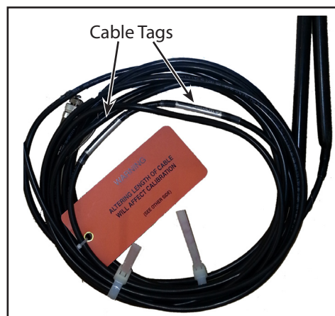
Figure 4. Cables with Cable Tags
