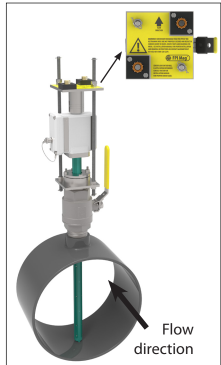
Figure 20. Meter oriented with flow direction
