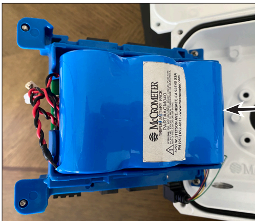
Large battery pack
