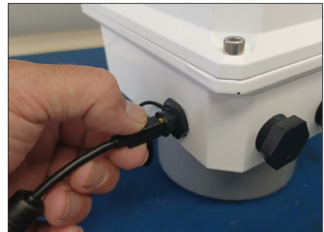
Figure 20. Plug in mini-USB cable
