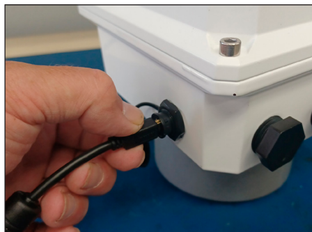
Figure 34. Plug in mini-USB cable
