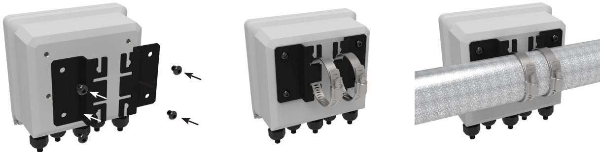
Figure 5. Mounting transmitter to horizontal post
