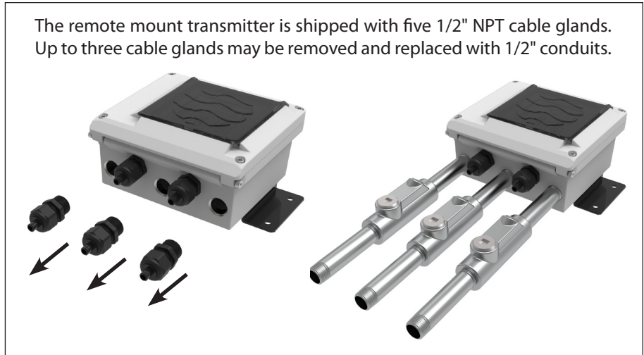
Figure 8. Remote mount transmitter with three conduit pass-throughs
