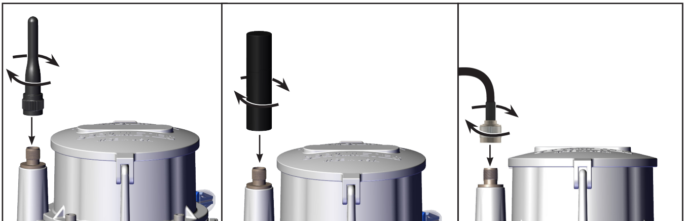
Figure 3. Attaching the cellular antenna
