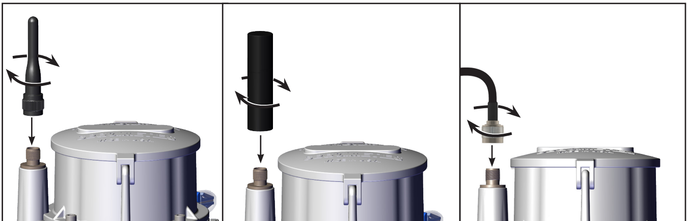
Figure 3. Attaching the cellular antenna
