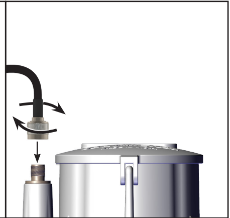
Figure 7. Attaching the antenna extension
