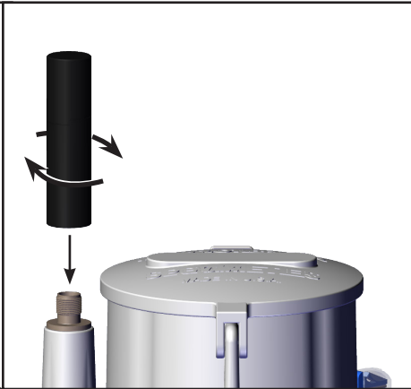
Figure 6. Attaching the satellite antenna
