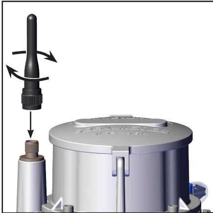
Figure 5. Attaching the cellular antenna
