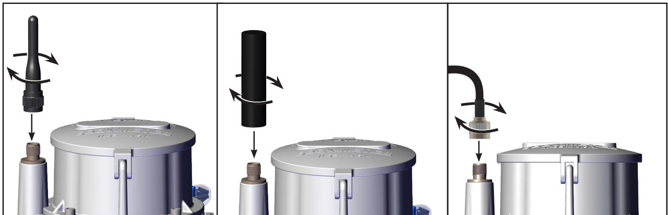
Figure 3. Attaching the cellular antenna
