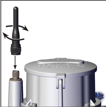
Figure 3. Attaching the cellular antenna
