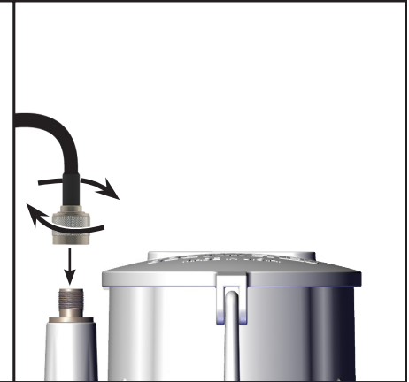
Figure 5. Attaching the antenna extension
