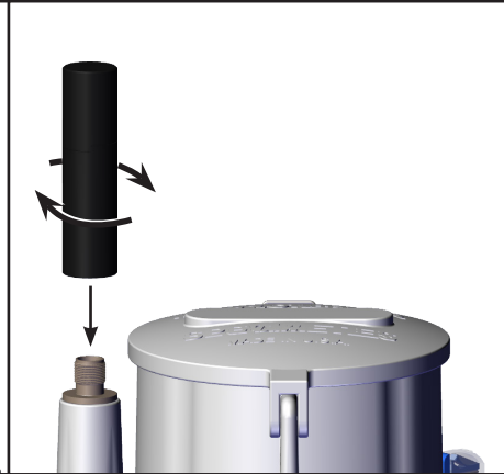
Figure 4. Attaching the satellite antenna
