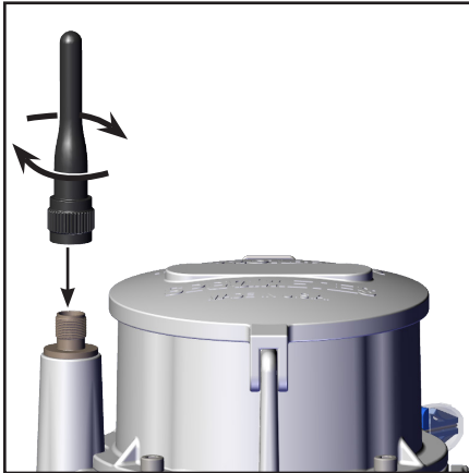
Figure 3. Attaching the cellular antenna
