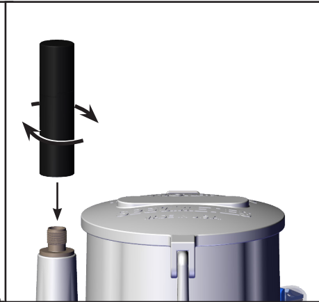
Figure 4. Attaching the satellite antenna
