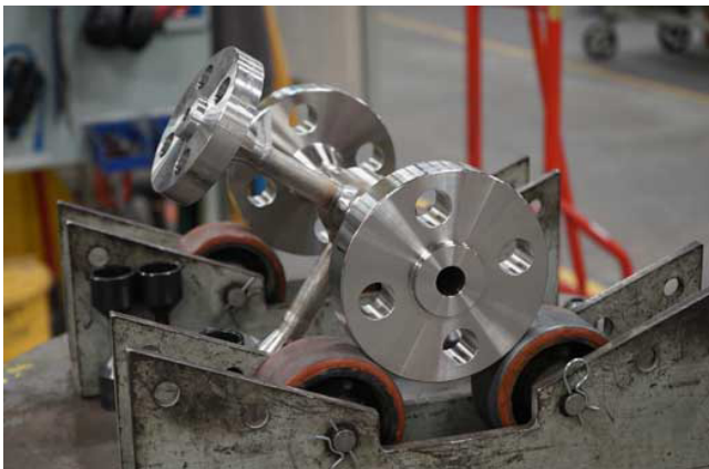
A V-Cone with flangeolet taps 90° apart to accommodate limited spacing
