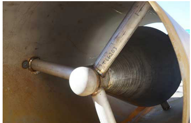
A view inside a large line size, 3-gusset V-Cone awaiting shipment
