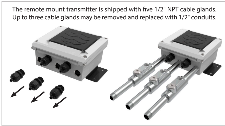
Figure 7. Remote mount transmitter with three conduit pass-throughs
